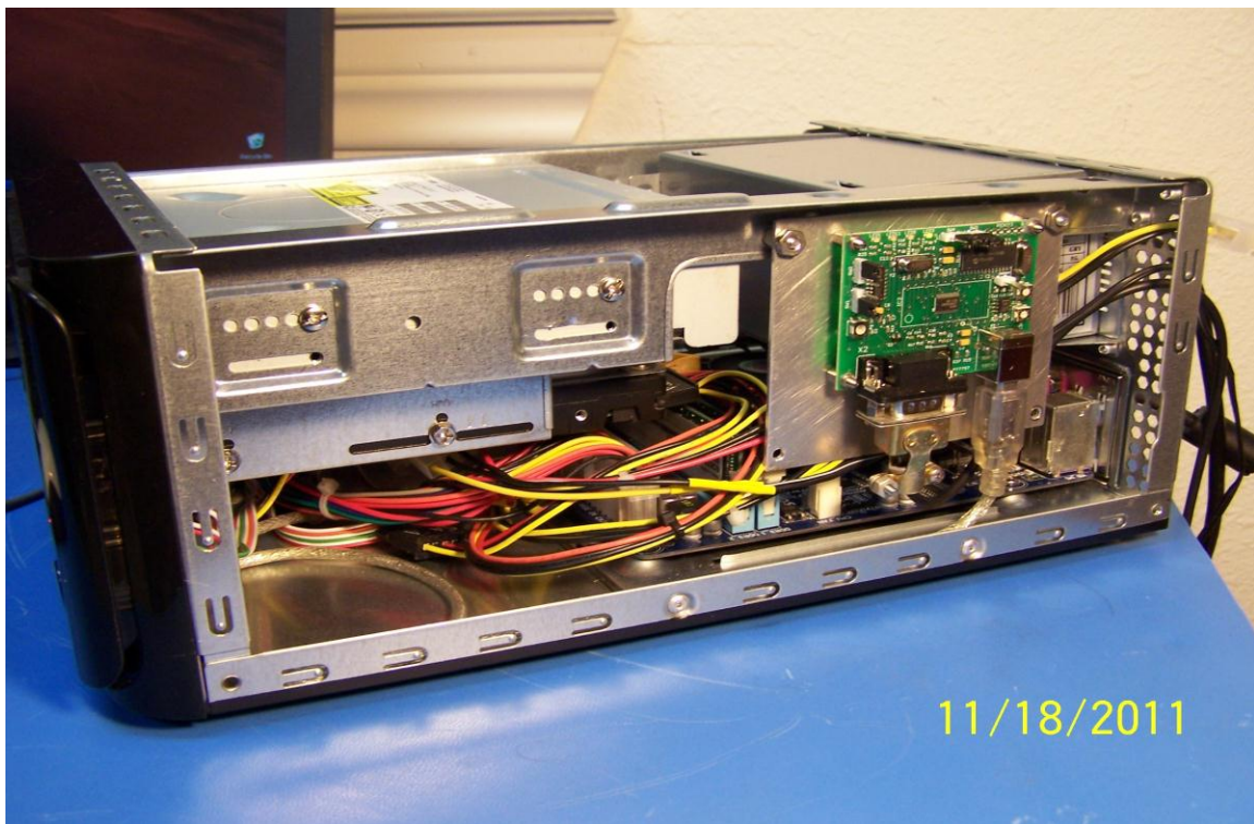
Side view of the computer, showing the Matrix Circuits StarBoard (Node Adapter) mounted inside, near the rear of the enclosure.
